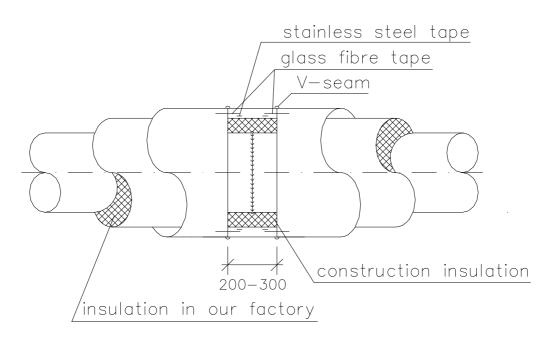
As soon as the insulation of the inner pipe has been finished, this area is once again to be protected in such a way that no water or dirt can penetrate into the ring space between the inner and outer pipes or into the on-site insulation; see also Sec. 2.2.3.
