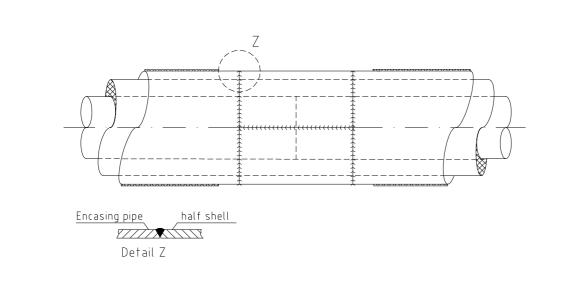
2.9.2 Joining encasing pipes by pulling together the encasing pipes
