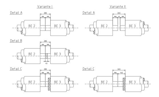
Expansion compensators in the form of elbows and Z bends are prestressed by the same procedure.
