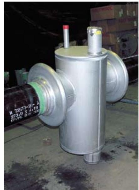
FW SAFETY PIPING for corrosive waste water: drainage point, inner pipe, encasing pipe and lenticular compensator made of stainless steel.
