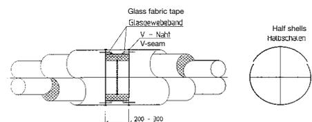
**Transitions between steel-cased and plastic-cased pipe-in-pipe without inspection chamber**
