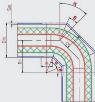
SIS pipe bend with multiple segments for large dimensions
