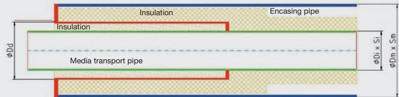
Bulkhead penetration with rigid connection
